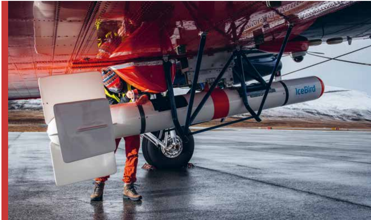
At Svalbard Airport near Longyearbyen, AWI sea-ice physicist Jakob Belter performs routine maintenance on the electromagnetic sea-ice-thickness sensor EM-Bird. Here the sensor can be seen in its specially designed cradle for take-offs and landings, which is mounted on the underside of the research aeroplane POLAR 6.
