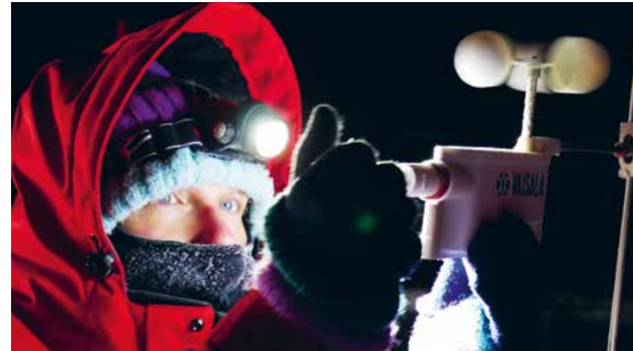
At the beginning of the drift experiment, US researchers erected a weather mast (l.) on the ice floe in order to measure the energy and heat flows in the air layers directly above the ice. In contrast, AWI expert Dr Anja Sommerfeld (top) focused on taking readings up to an altitude of roughly 30 kilometres.
