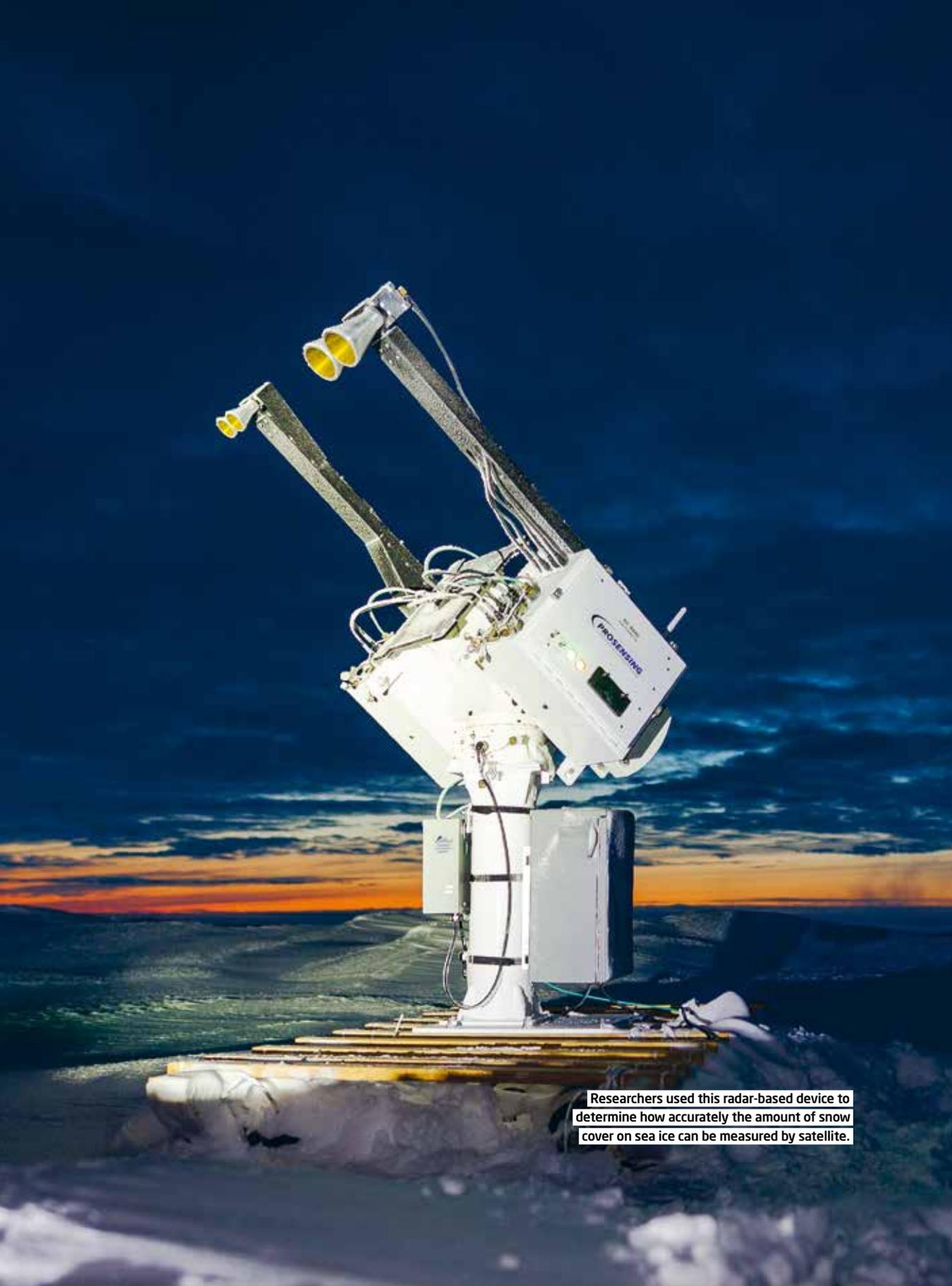
Researchers used this radar-based device to determine how accurately the amount of snow cover on sea ice can be measured by satellite.
