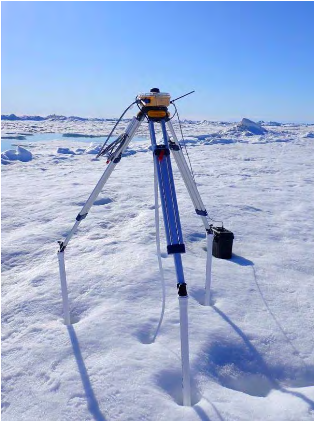
Fig. 2 Figure 3: A digital thermistor chain unit in the old Central Observatory on 21 July. (Photo: Ilkka Matero)
