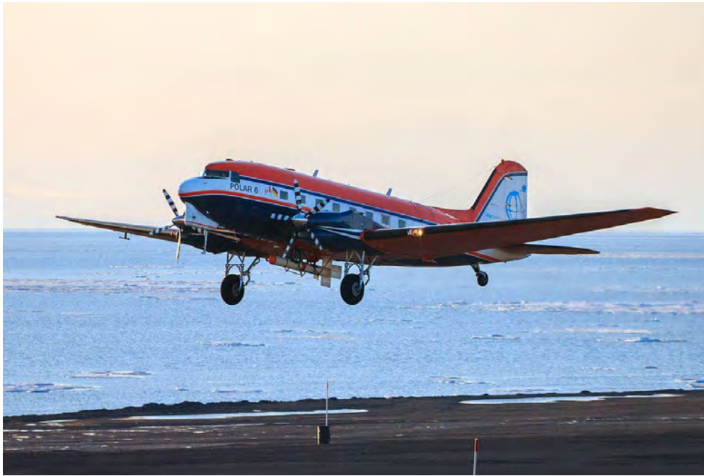
Image 1: The polar aircraft Polar 5 and Polar 6 can be fitted with a torpedo-like electromagnetic sensor, the EM-Bird, which is stowed away in a 'nest' on the ship's underside for take-off and landing. Once over the sea ice, the sensor is towed behind the plane on a 70-m-long cable, measuring the thickness of the ice from a height of 15 metres above its surface (photo: Jan Rohde, AWI).
