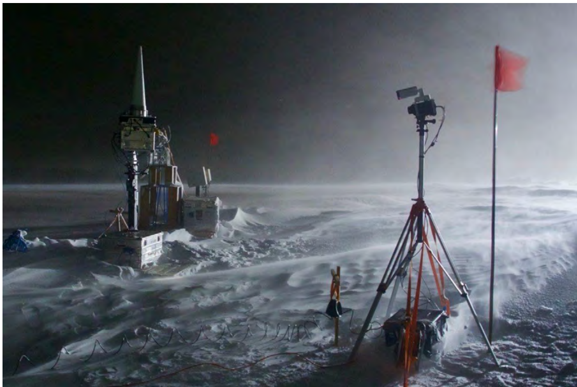
Equipment used to monitor and determine the microwave characteristics of the snow and ice conditions in the vicinity of the MOSAiC ice camp (Photo: Gunnar Spreen / IUP Bremen).
